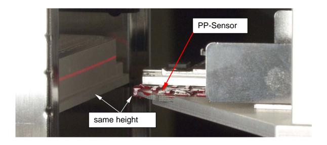
"This adjustment has to be done after the adjustments for the transfer of plates from/to the cassettes."
