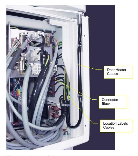
The door heater cables are marked as follows:
